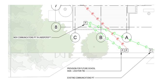
**Power:** Proposed power supply will be an underground cable from a new private pit established within the property boundary adjacent the existing Essential Energy pole 15749. A new underground cable will connect this private pit to the new main switchboard:
